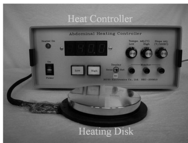
Figure 1. HTCD is composed of a heating disk, temperature sensor and a heat controller.
